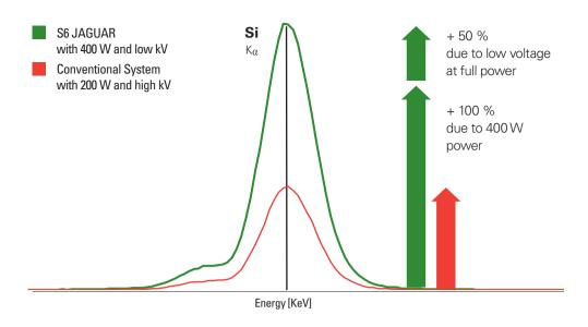
S6 JAGUAR offers about 3 times more intensity due to optimized exitation with low voltage at full power
