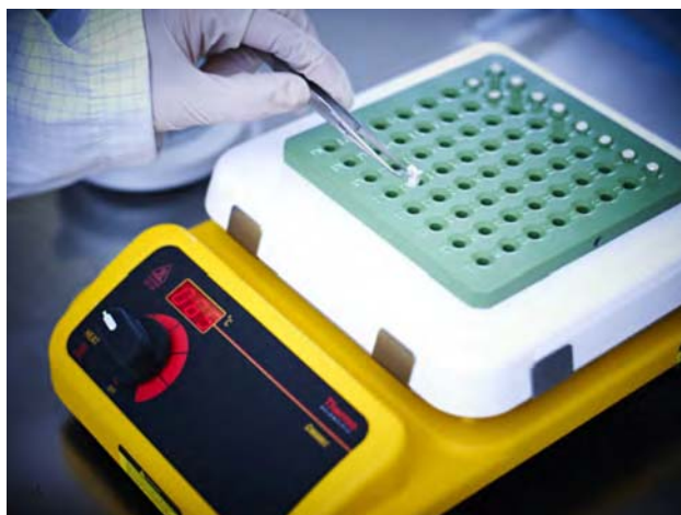
Figure 17-1. Sample Holder Plate and Electric Heater
