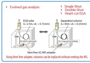
Switching between EGA tube and separation column
