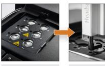
The sample vial is incubated/agitated to speed up analyte equilibration.
