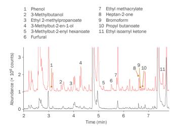
Sample stacking (red trace) greatly increases the number of important trace-level aroma compounds identified in this headspace-trap analysis of orange juice.
