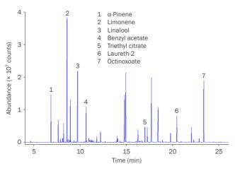
Valuable information about the semi-volatile components (5–7) in this fragranced shower gel is obtained by using immersive high-capacity sorptive extraction. Headspace would have given much lower responses for these compounds.
