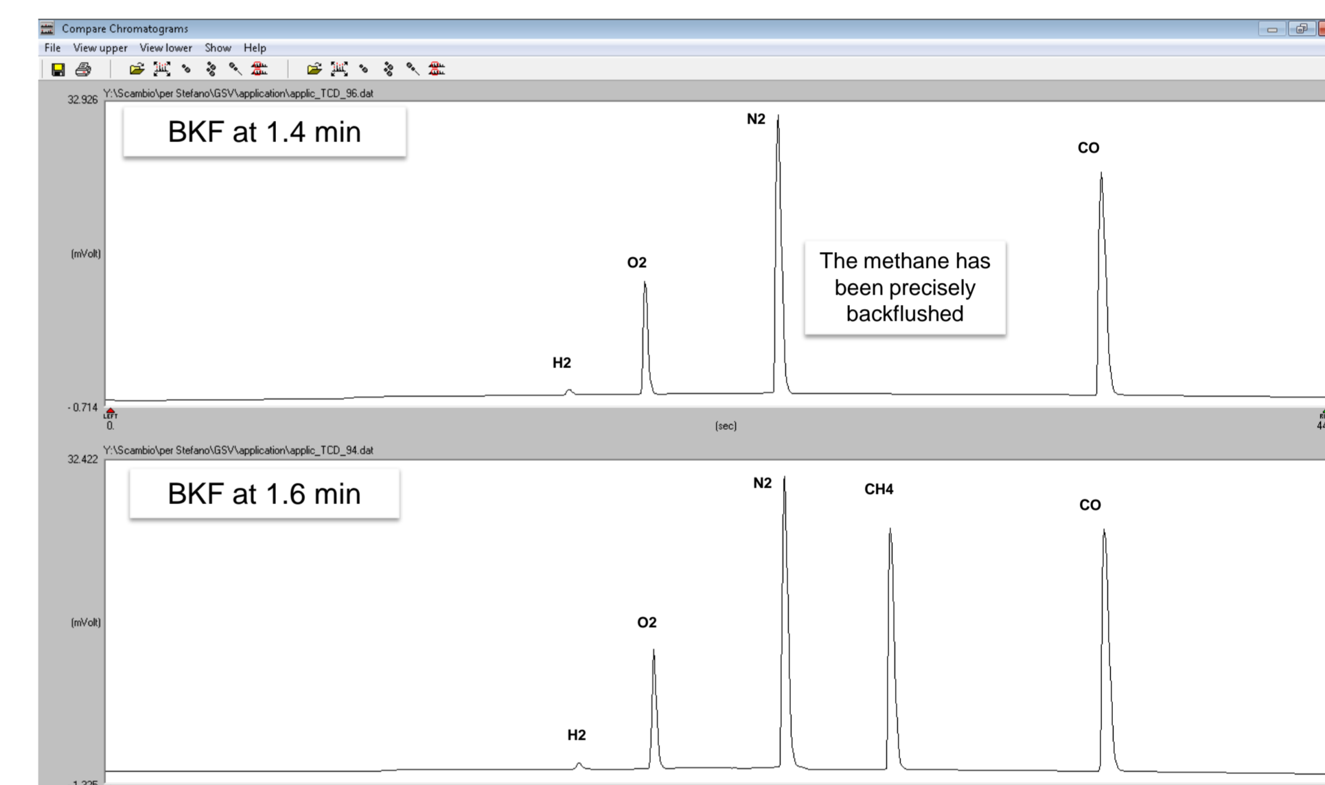
FIGURE 5. Selectivity of the back-flush cutting.
