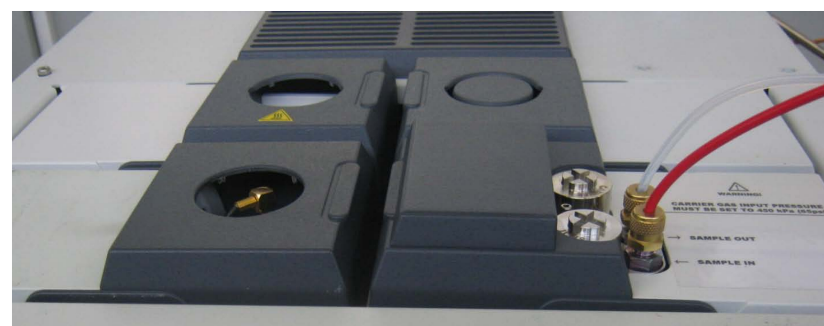
FIGURE 2. TRACE 1300 equipped with GSV module and FID-TCD in series
