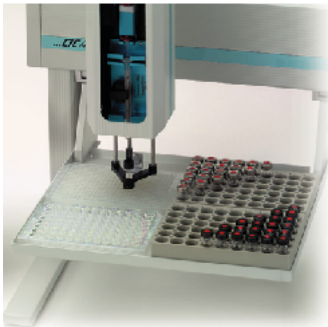
Flexible utilization of microplates with 2ml vials on the same Trayholder
