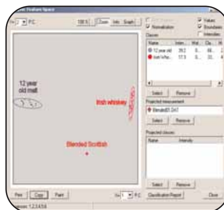
Aroma profiling of whisky vapours with e-nose showing differentiation of whiskey types
